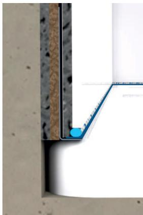
Application of the joint filler to protect the seal in case of later replacement.
