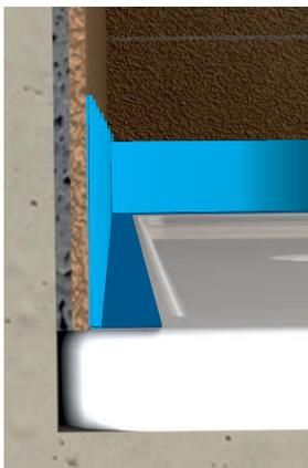
The tub top sealing tape is applied to the tub and existing surface.
